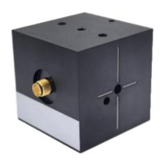
Goptica's Phase Modulators use a variety of electro-optical crystals such as MLN, DKDP, KTP, LT, etc. The wavelength covers 350-3000 nm, the frequency covers 1-4 GHz, and the modulation depth is up to 2  $\pi$  rad.
